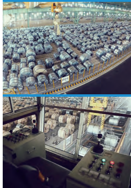
▲ The unmanned traveling crane is lifting the steel coils
